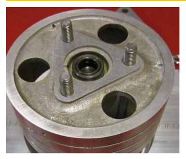
Fig 1 Slip the Thin Spacer Plate (1/8") over bolts as shown
