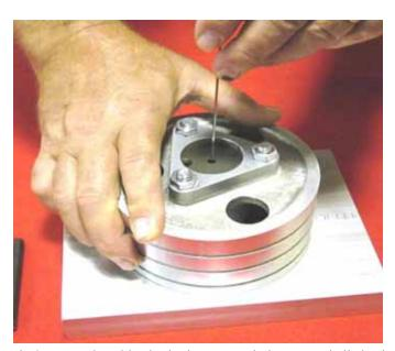
Fig 3 Insert clean bleed-wire into center hole to open ball check in the lifter unit below.
