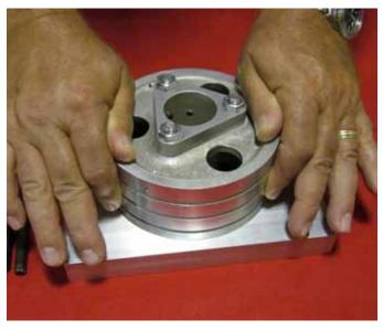
Fig 4 Verify that all air is removed from Hydraulic unit. If it is properly filled and bled, it will feel like it is stuck or locked up.
