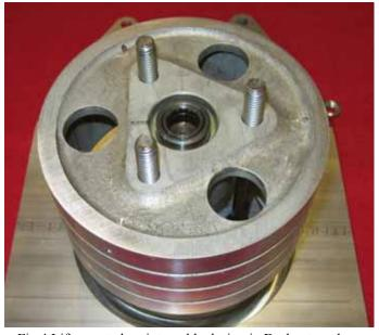
Fig 4 Lifter seated on internal lock ring in Dashpot as shown
