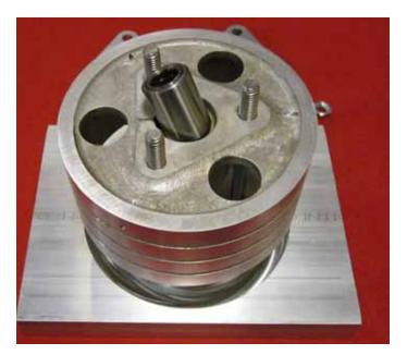
Fig 3 Slip lifter into Dashpot as shown
