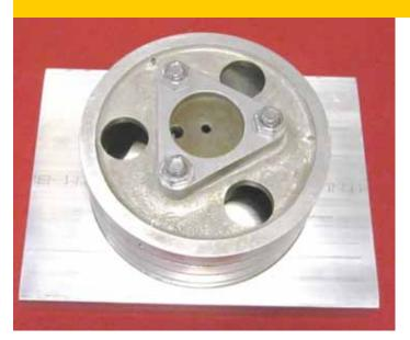
Fig 1 Remove the hex rods and place onto fixture as shown
