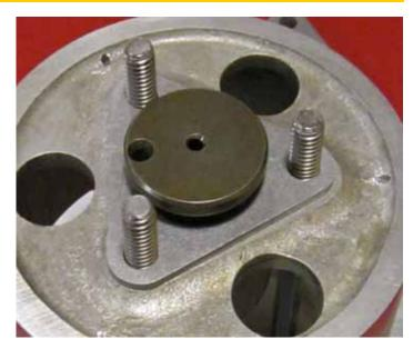
Fig 2 Place Driver into lifter as shown
