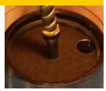
Fig 2 Overfill lifter & cavity thru center hole with clean oil
