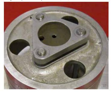
Fig 3 Slip Driver-Capture Plate over bolts as shown
