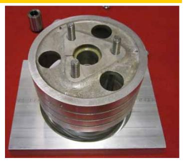
Fig 2 Slip Dashpot over bolts as shown
