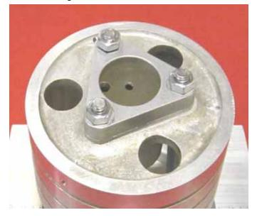
Fig 4 Screw lock-nuts on bolts (deformed thread UP) as shown
